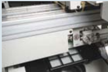
Loader capacity: \phi 50 mm x L 50 mm, 0.5 kg x 2 Max. Feed rate: X-axis 180 m/min Y-axis 130 m/min Z-axis 55 m/min
